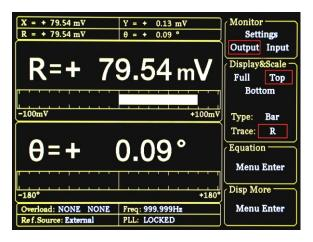
In X-Y chart, OE1022 shows the trend of measurement results over time, and check the value by using knob control cursor
